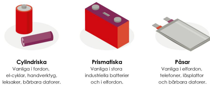
Figure 2. Appearance and presence of lithium-ion batteries.
