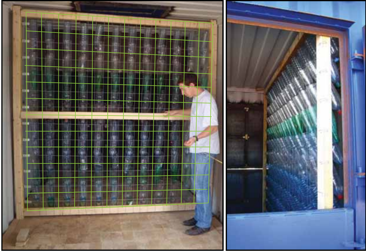
Figure 19. The "bottle frame" in the non fire part of the compartment
