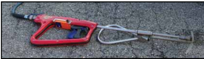
Figure 3. Hand held part of the nozzle, with two triggers; one for water and abrasive, the second only for water. Picture: Service communication SDIS68
