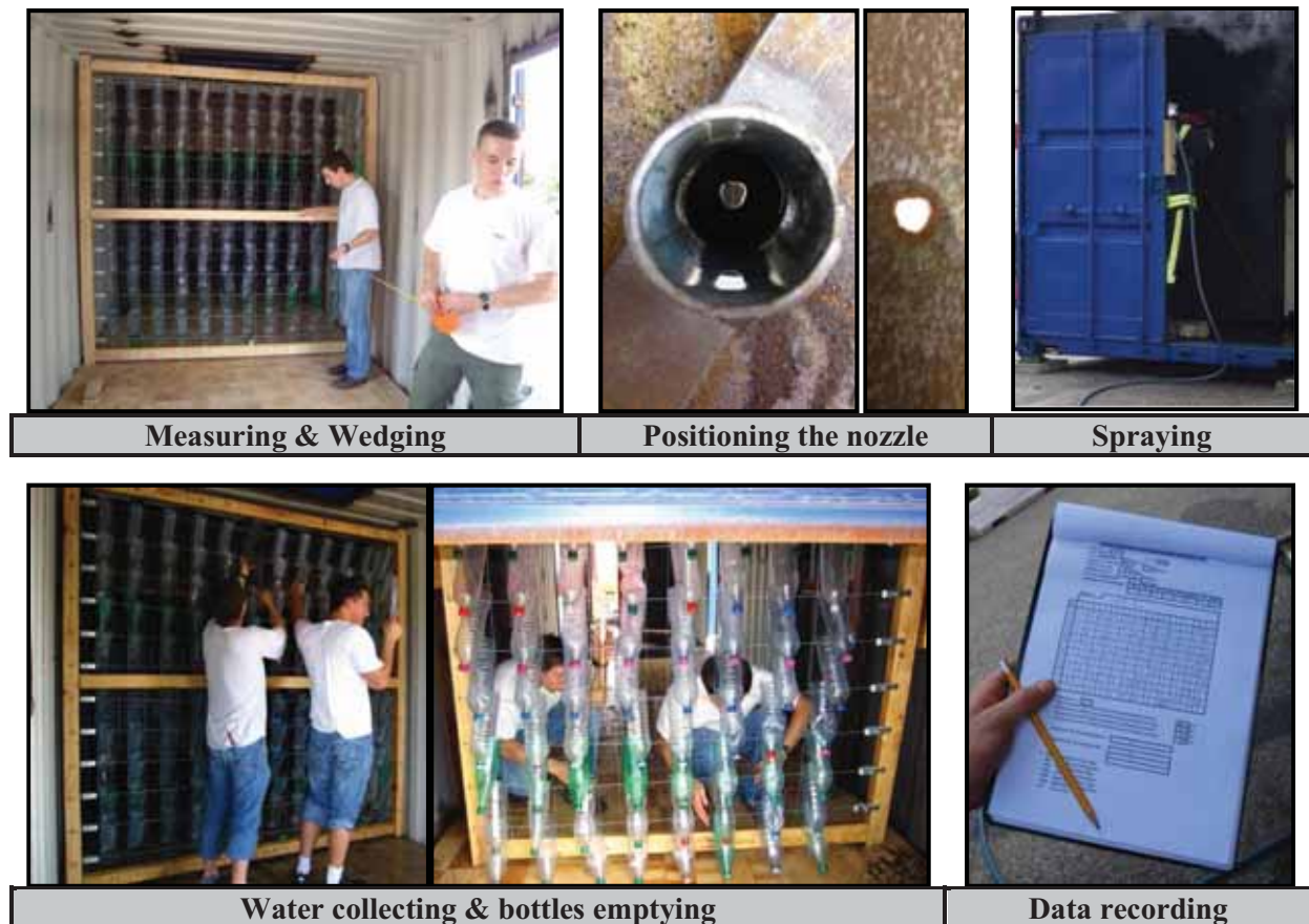
Figure 29. Water mist flux density measurement protocol
