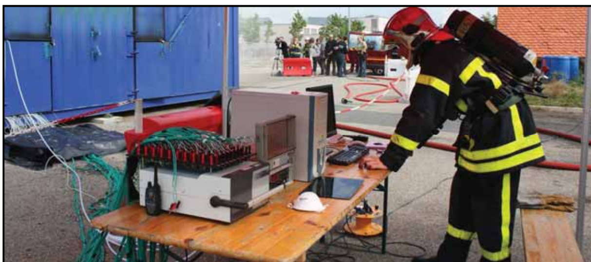
Figure 22. TC network, running from the compartment to the data logger. Picture: Service communication SDIS68
