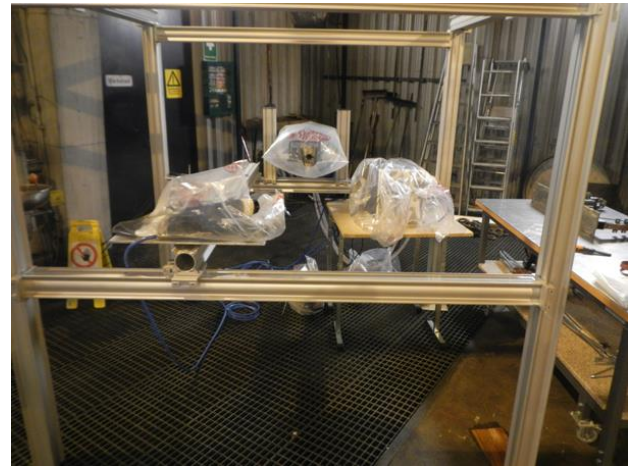
Figure 3: Water proof implementation of the laser diagnostic drop sizing. The aluminum cage was also covered by a tarpaulin, not shown here.
