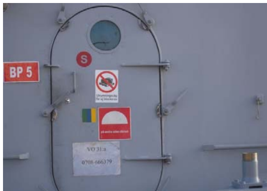
Figure 4 Cutting extinguisher Attack Point "S" at a hatch; CAP adopted by Greater Gothenburg Fire and Rescue Service
