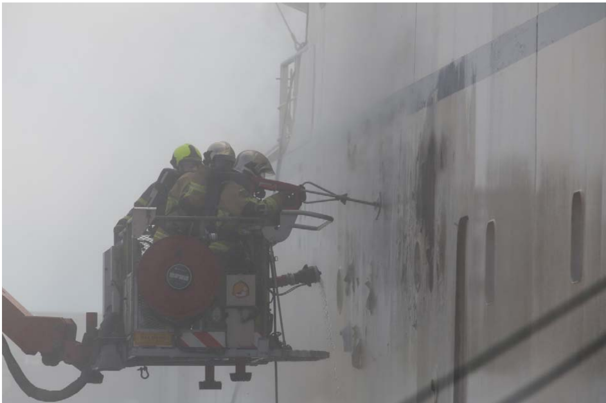
Figure 13 Cobra Cutting Extinguisher applied by Amsterdam Amstelland Brandweer from an aerial ladder on the SCH 118
