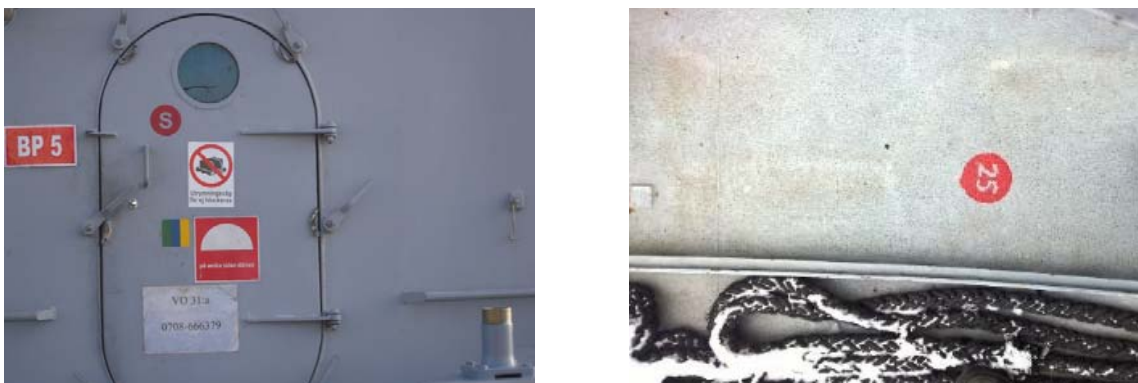
Figure 5 Cutting extinguisher Attack Point “(S)” at a hatch and “(25)” on deck, photos courtesy Royal Swedish Navy
