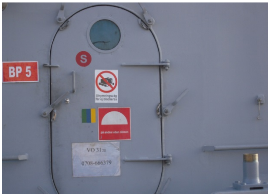
Photo 3, Cutting extinguisher Attack Point "(S)" at a hatch and "(25)" on deck (Royal Swedish Navy)
