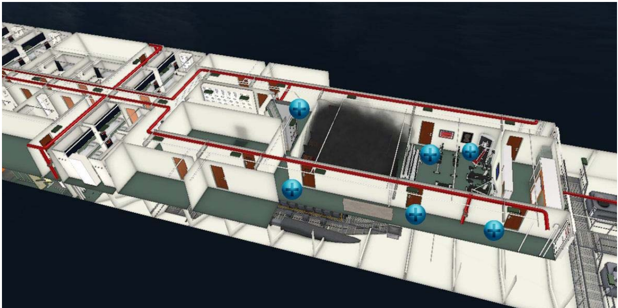
Figure 8, Defensive pressure ventilation, principal sketch
