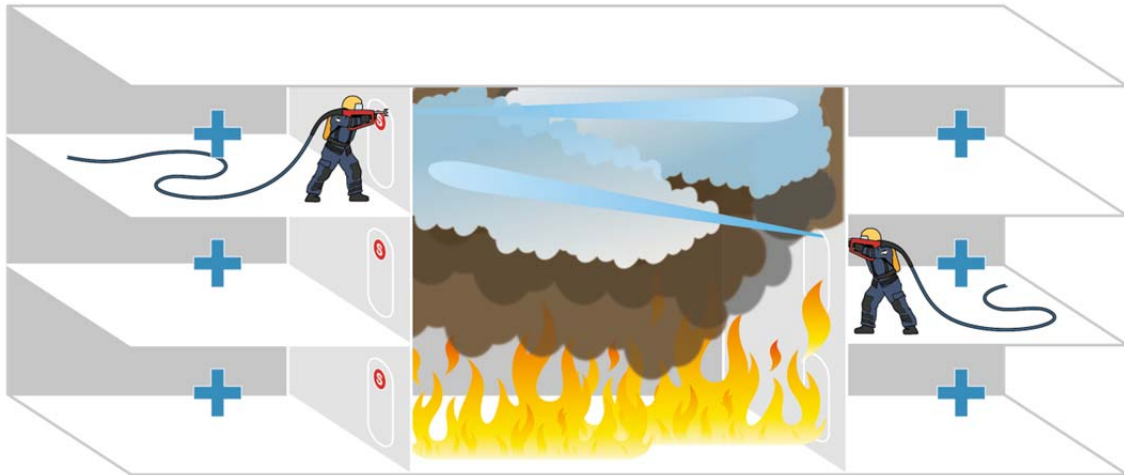
Figure 14, Step 2, Cool fire gases, continue isolation
