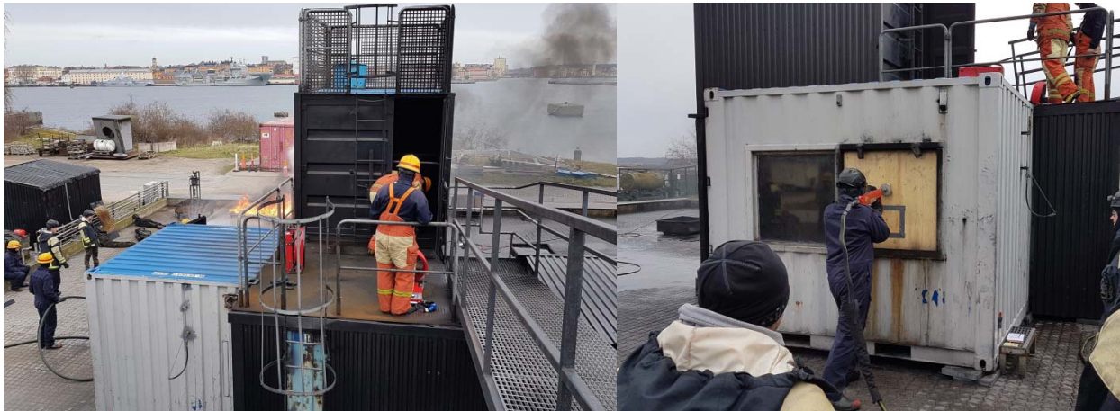
Photo 9, Engine room annex - vertical positive pressure ventilation with external gas cooling (Cobra)
